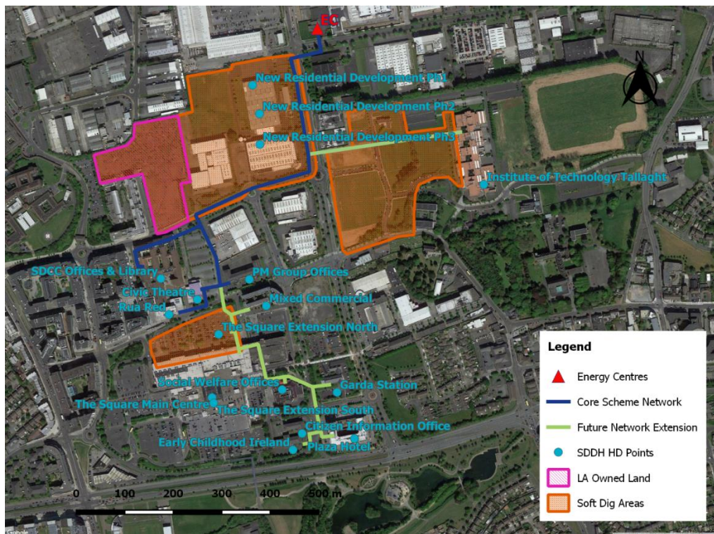
Figure 25: Resulting Preferred Network Route
